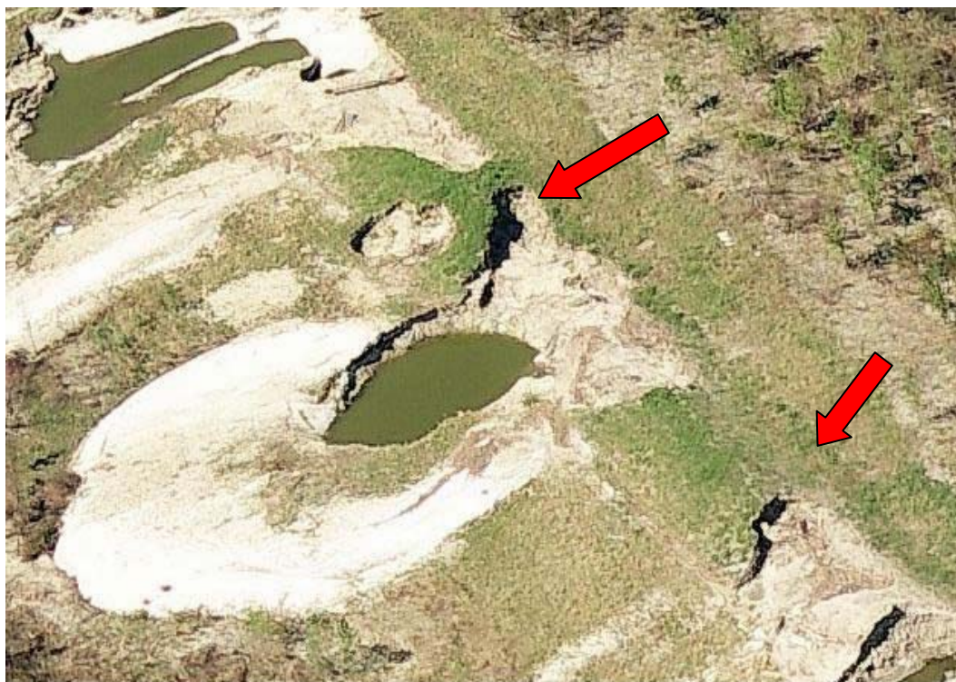
Figure B-15. High resolution pictograph of Reach 2 EBSBs showing wave erosion features (photograph provided by Dr. Paul Kemp).
