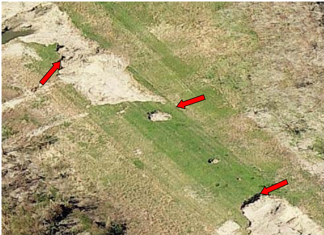
Figure B-14. High resolution pictograph of Reach 2 EBSBs showing wave erosion features (photograph provided by Dr. Paul Kemp).
