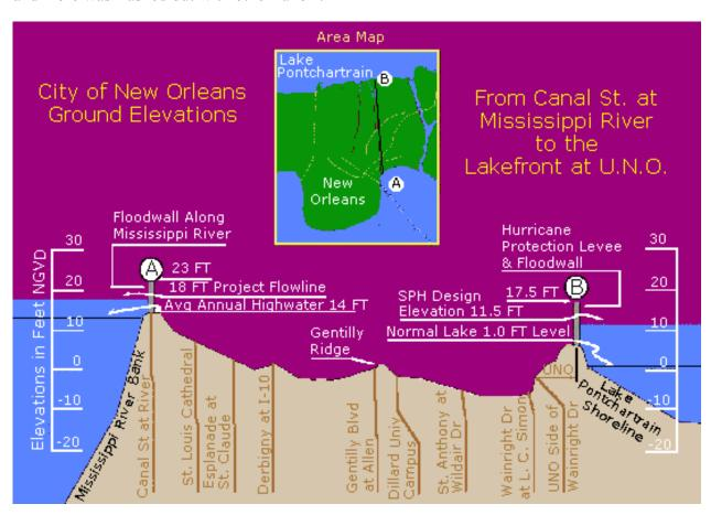
Figure 6. Cross section of New Orleans proper showing elevations
