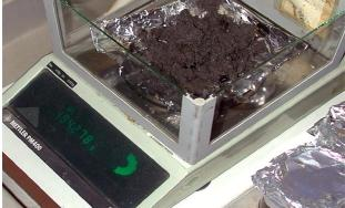
Figure 9. Removing and weighing sediment
