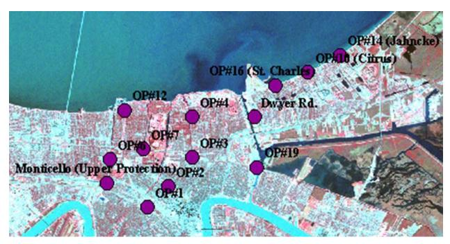
Figure 3. Locations of pump stations for Orleans Parish included in the model that pump into the lake
