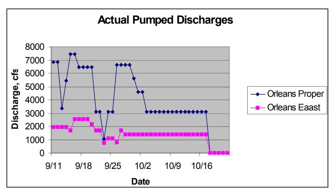
Figure 2. Time series of combined *actual* pump discharges for Orleans Proper and Orleans East that pump into the lake
