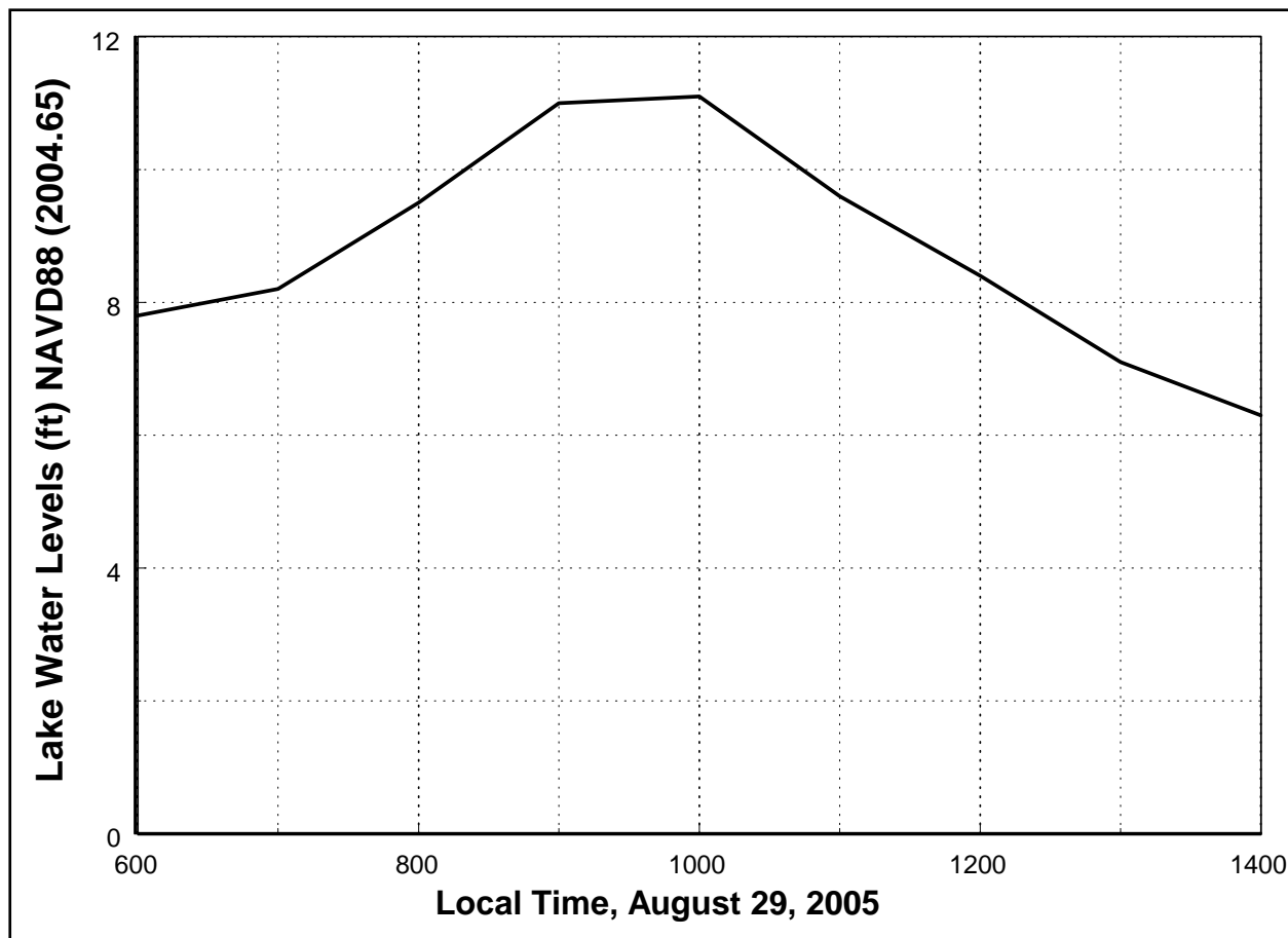
Figure 11-4. Estimated water levels in Lake Pontchartrain near north end of London Avenue Canal
