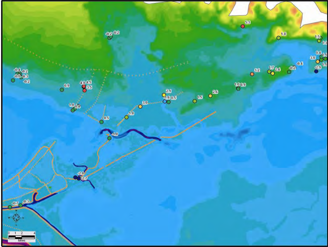
Figure 5-13g. Topographic contours (ft) and HWM elevation errors (ft) with the error value (ft). Detail of Orelans Parish and Slidell, MS
