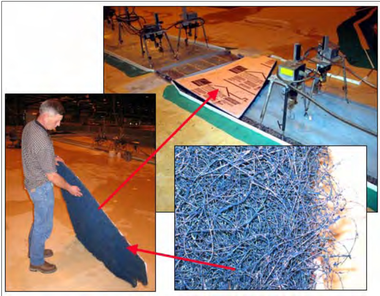
Figure 12-20. Debris field simulation using fiber mesh material
