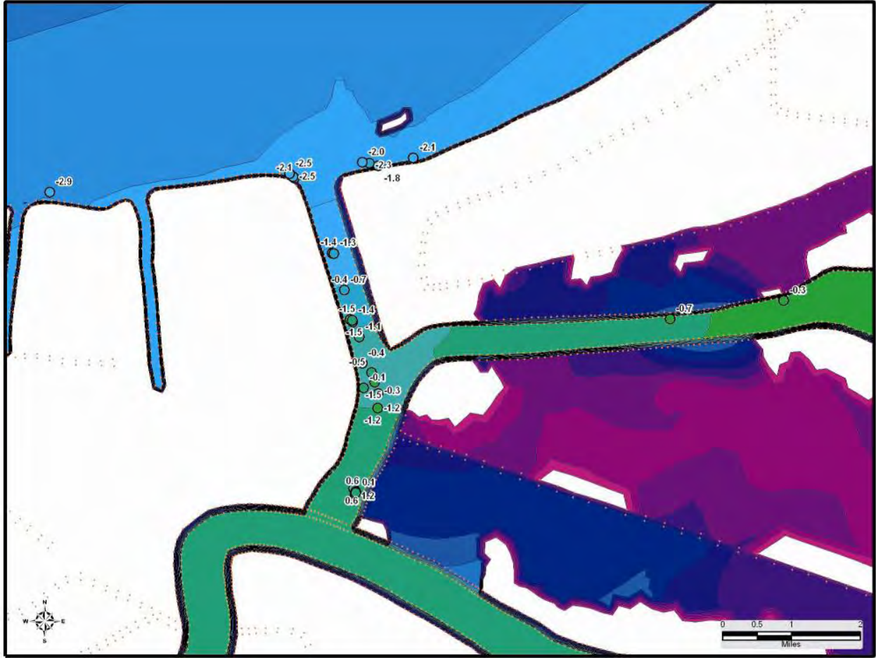
Figure 5-12d. Modeled maximum event elevation contours and HWM elevations in circles (ft NAVD 88 2004.65) with errors (ft). Detail in the vicinity of the GIWW and IHNC
