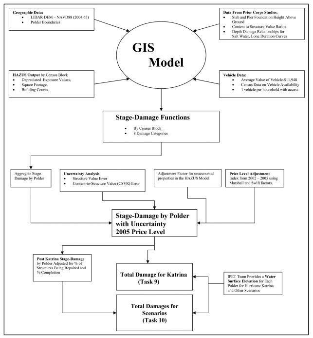
Figure 1-2: Flow Chart of Flood Damage Calculations in GIS-based Model
