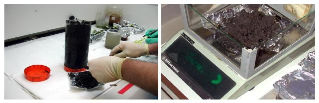
Figure 9. Removing and weighing sediment
