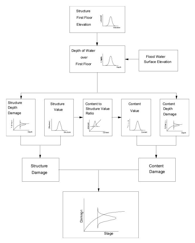
Figure 1-5. Example of Typical Corps Approach to Uncertainty in Stage-Damage
