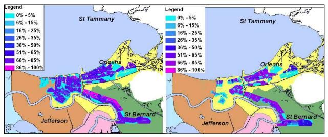
Figure 1-4. Percent of Property Damaged--Comparison of Model Results for Katrina Flooding (left) and Hypothetical Scenario #2, Resilient Levees and Pumps (right)
