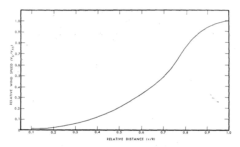
Figure C-12. Variation of relative wind speed with relative distance within the radius of maximum winds for the stationary SPH and PMH. (item 57 of Appendix A)
