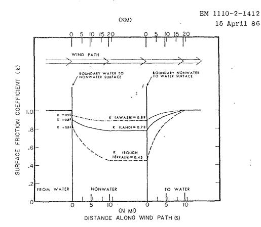
Figure C-15. Schematic of near shore frictional adjustments. (item 57 of Appendix A)
