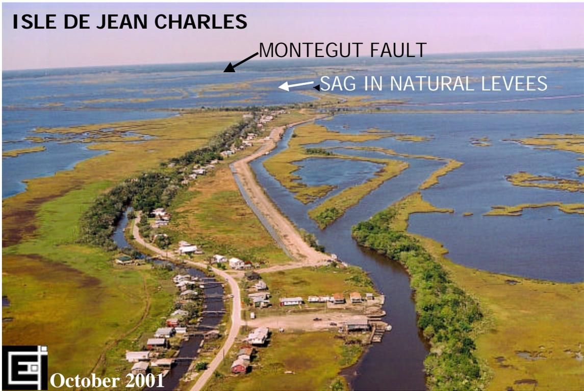
Figure 54. Looking north along Isle de St. Jean Charles. The severed natural levee ridge along the bayou can be seen in the background. Part of the ridge has been submerged as a result of fault movement. Photograph by S.M. Gagliano, October 17, 2001.
