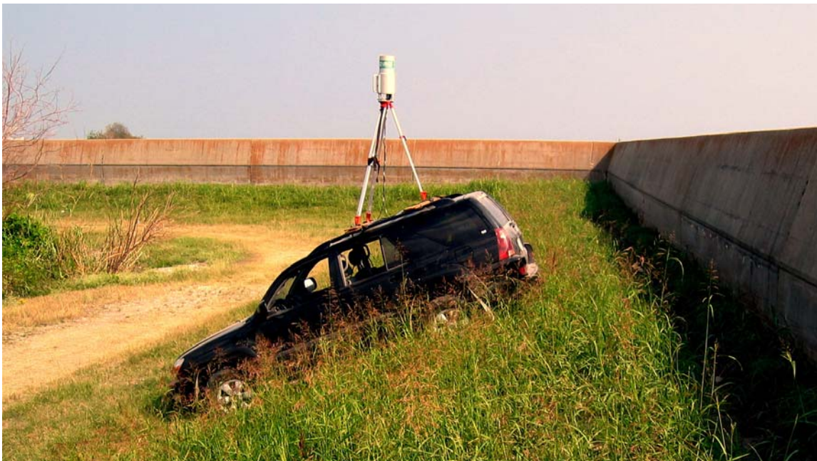
Figure A-2: Entergy Plant I-Wall scanned using the USGS Coastal and Marine Geology Team terrestrial LIDAR unit and tripod mounted to the roof of our field vehicle. The fixed roof base allowed for the leveling of the tripod and LIDAR instrument on sloping ground.
