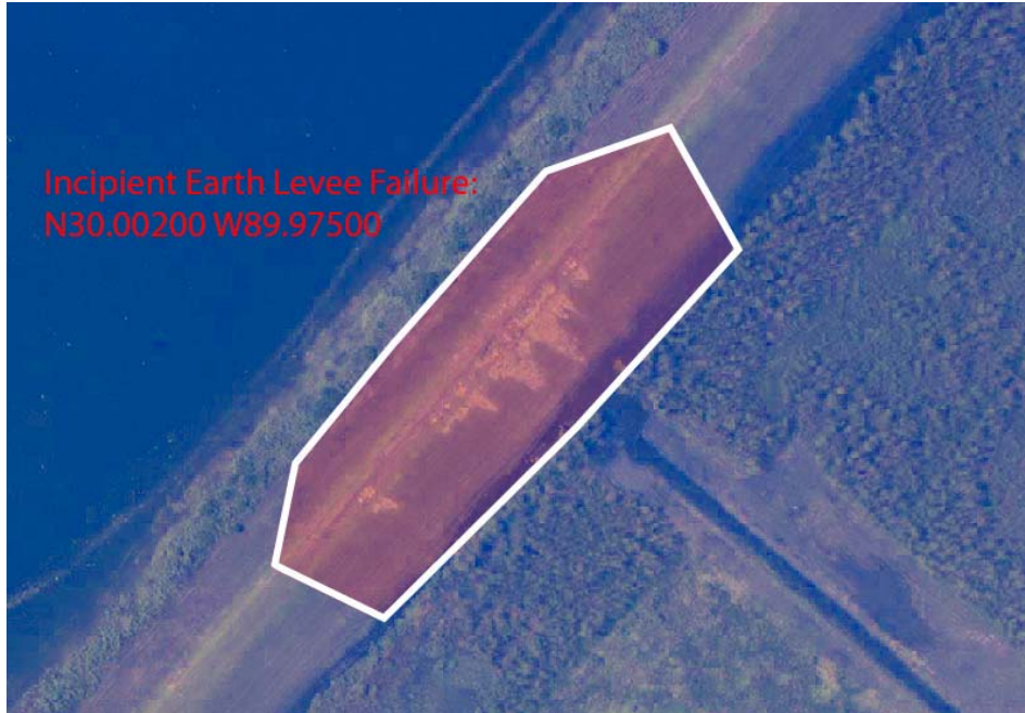
Figure A-11: Site 9, Earthen Levee Section Distressed by Overtopping Erosion at N30.00200°, W89.97500°
