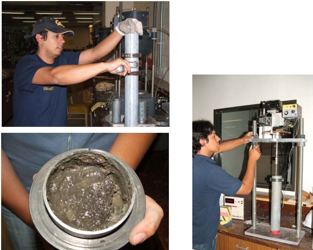
Figure E-1: Laboratory vane shear testing of the thin layer of sensitive organic silty clay
