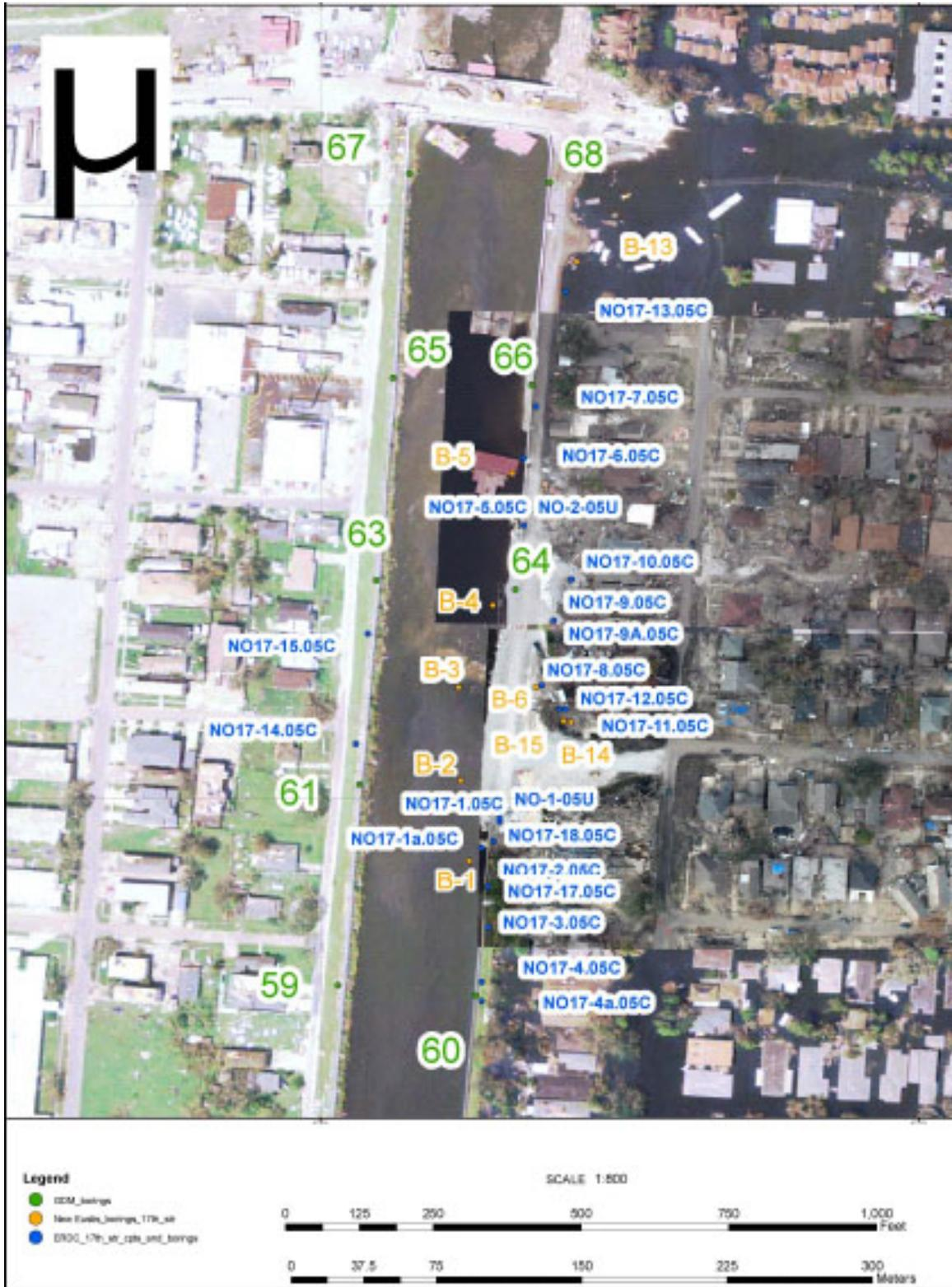
Figure 25(a): Plan view of 17<sup>th</sup> Street Canal showing locations of IPET borings and CPT
