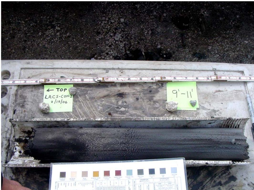
Figure 8.109(a): Sample across transition zone at London Avenue Canal, South Breach Section
