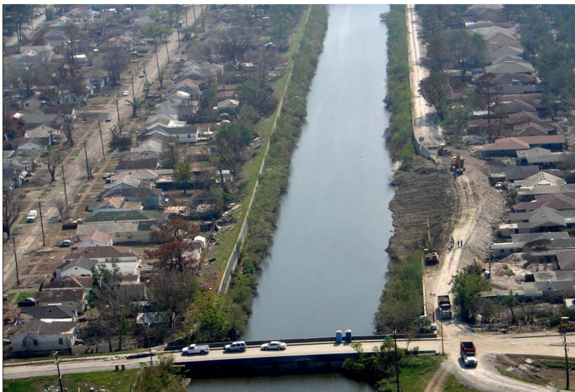
Figure 8.111: Oblique aerial view of the breached section on the west bank of the London Avenue Canal (North) and the “distressed” section on the east bank (on the left in this photo, which is taken looking to the south.)
