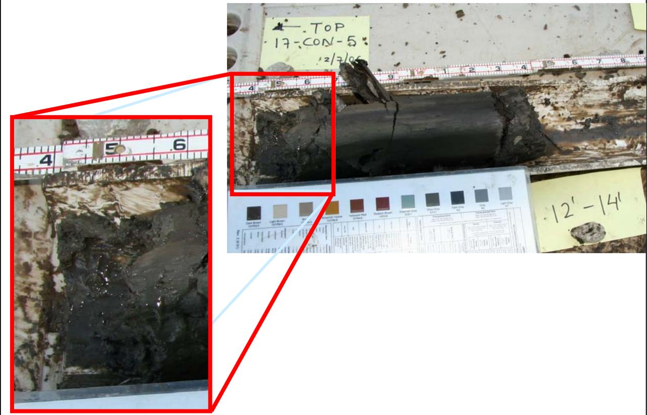
Figure 8.54: Photo of an “undisturbed” sample of the sensitive organic silty clay.
