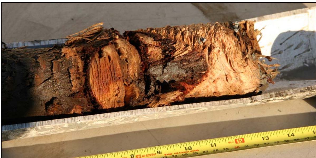
Figure 3.15: Wood and other organic debris was commonly sampled in exploratory borings carried out after Hurricane Katrina throughout the city. This core contains wood from the old cypress marsh that was recovered near the 17 th Street (Metairie Relief) Canal breach. Organic materials are decaying throughout the city wherever the water table has been lowered, causing the land surface to subside (photo by C. M. Watkins).
