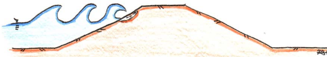
Figure 10.5: Wave impacts can cause significant erosion to levee faces. Wave-induced erosion consists of run-up (sloshing up and down of water as a result of staggered wave arrival) and “mini-jetting” when the crest of the waves breaks on the levee face.
