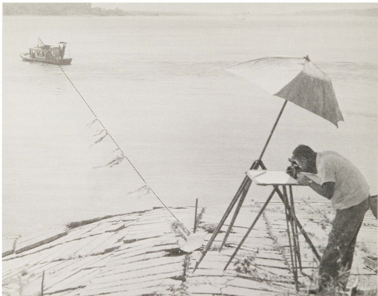
Figure 8. Radial-arc survey procedures with sounding boat, distance wire, and plane table
