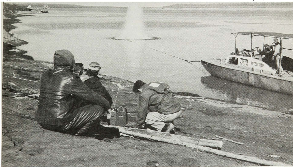
Figure 34. Subaqueous seismic refraction test
