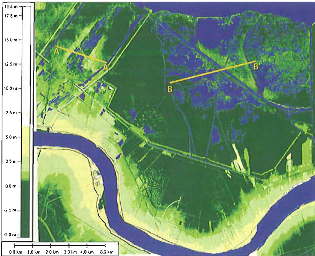
Figure 3. Digital LIDAR elevation map showing elevation (NGVD 1984) in the Bonnet Carre spillway and the LaBranche wetlands displayed using Global Mapper 9.0 (Day et al. 2012).
