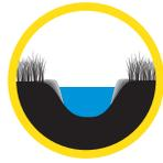
**Bank Stabilization** is the onshore placement of earthen fill and vegetation planting designed to reduce wave energies and maintain shorelines in open bays, lakes, and bayous, including navigation channels.
