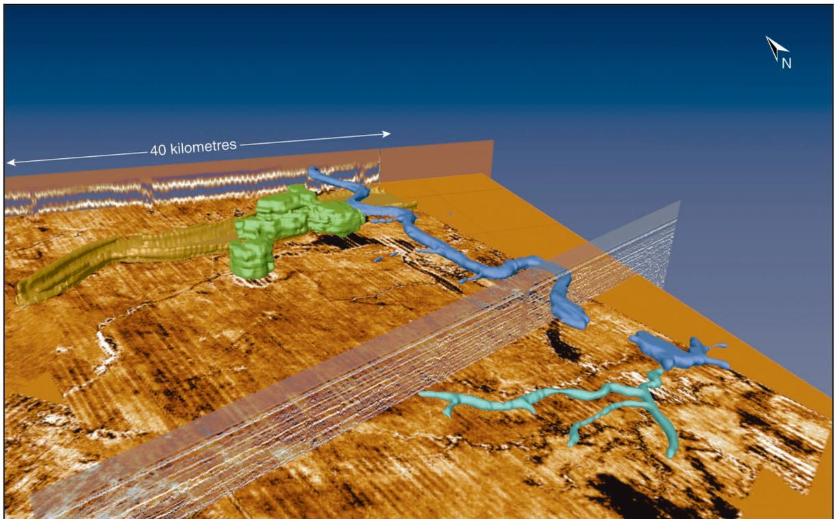
Figure 5.14 Seismic data cube illustrating chronostratigraphic relationship between the meandering Holocene river, now named the Shotton, and earlier features
