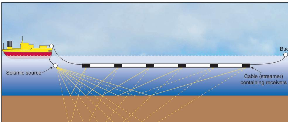
Figure 3.3 Typical marine seismic reflection acquisition
