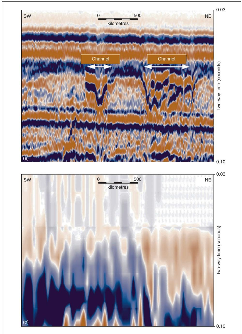
can be converted into an approximate depth and the continuous record built up into a profile through the Earth's surface. Typically, a vessel towing an acoustic source collects seismic data through a series of hydrophones designed to record the reflection from the seabed.
