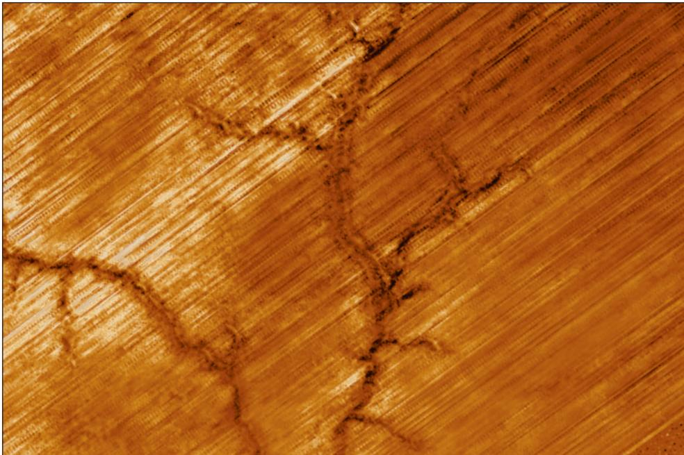
Figure 3.16 An extremely clear image of a submarine palaeochannel in the North Sea study area. The actual river channel can be seen as a dark line inside the river valley
