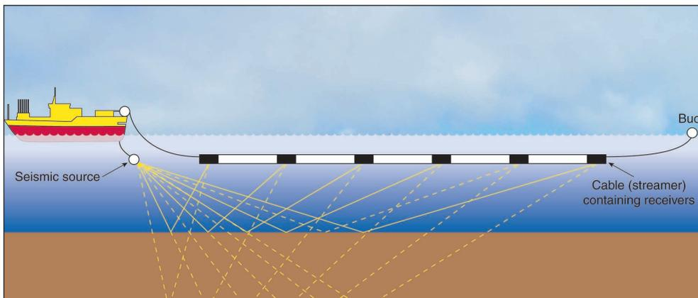
Figure 3.3 Typical marine seismic reflection acquisition
