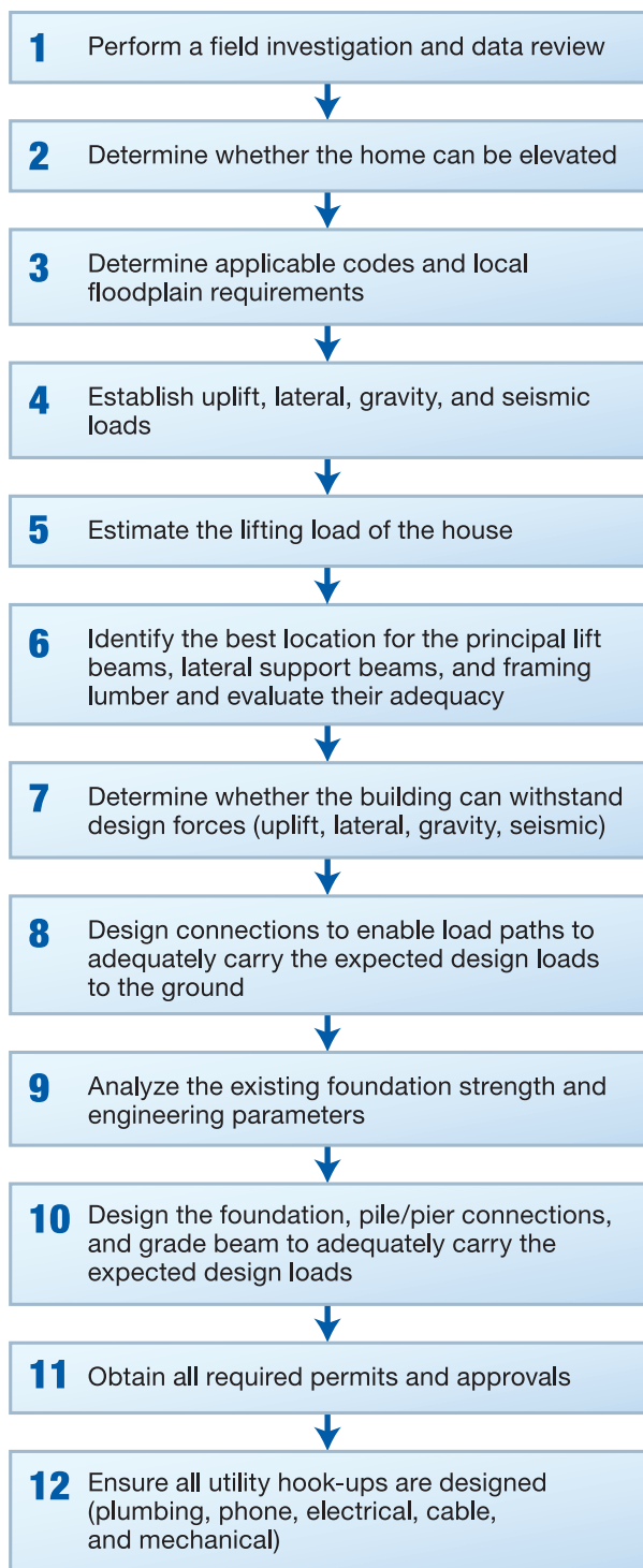
Figure 9: 12-step design process for elevating homes
