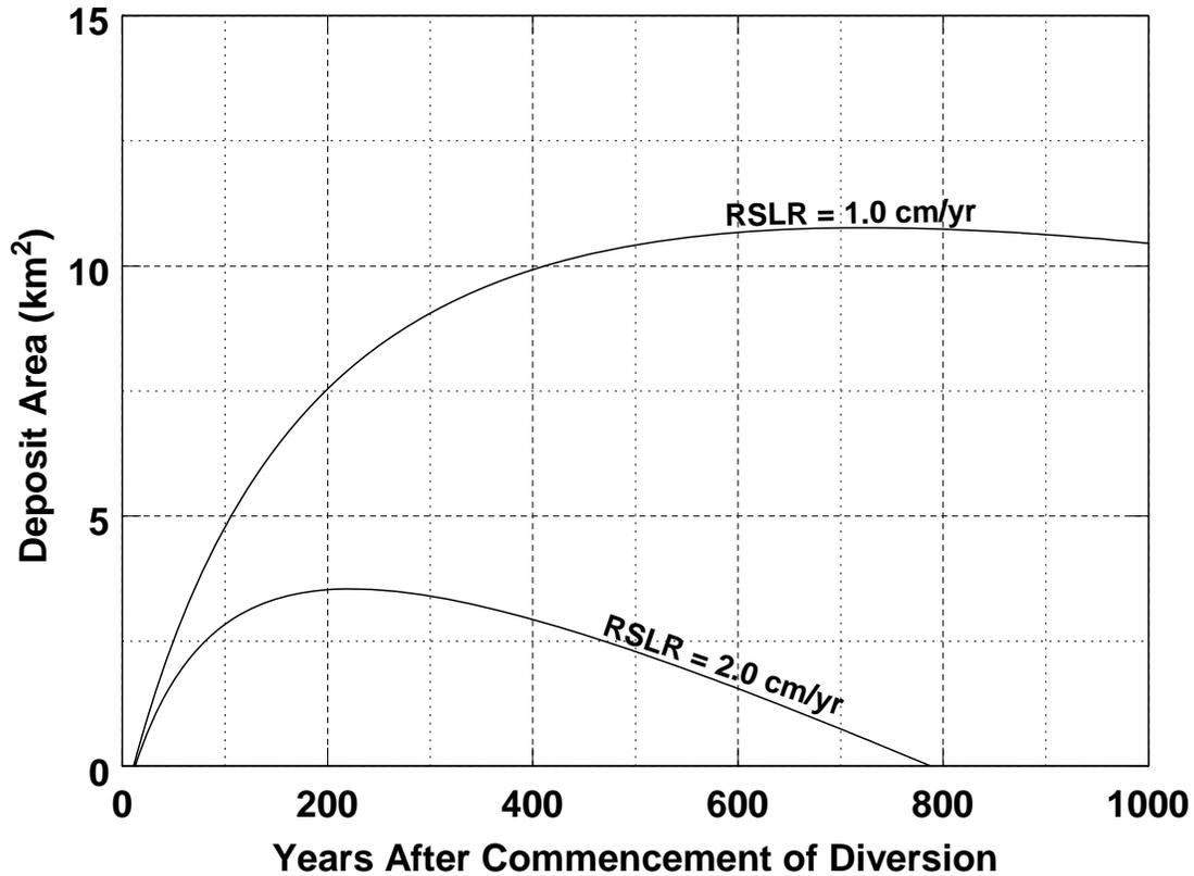
Figure 13. Example 5. Comparison of subaerial areas over time for relative sea level rise rates, uniform width = 2,000 m, annual retention of sediment = 200,000 m<sup>3</sup>/yr. Initial depth of receiving waters = 2.0 m, elevation of horizontal portion of deposit above mean water level = 0.25 m, foreset slope = 0.002, bottom slope = 0.
