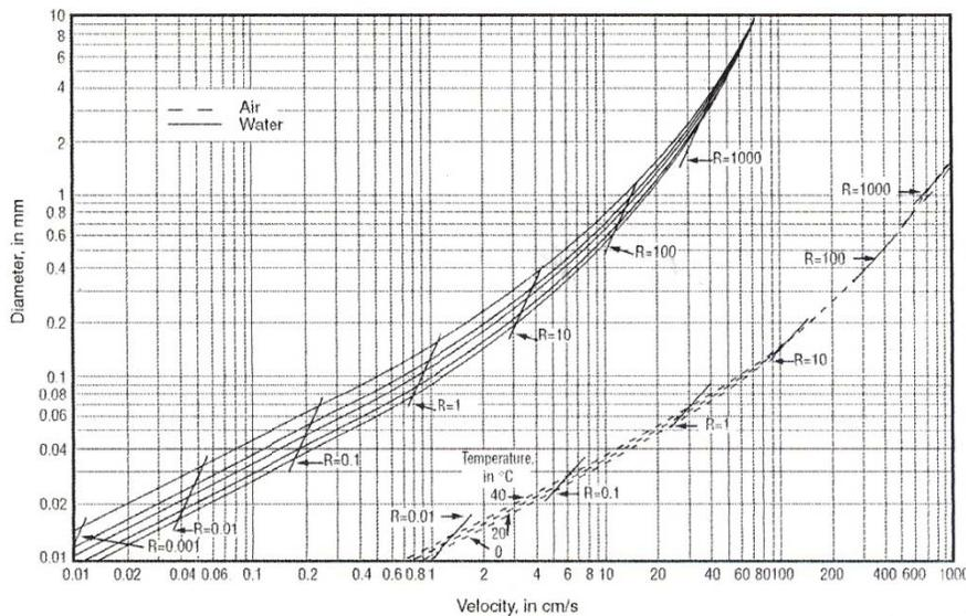
Figure 3. Fall velocity vs. sediment diameter (Rouse, 1937)
