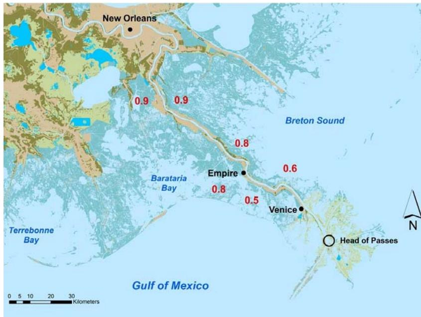
Figure 15. Preliminary recommendations for proportion of diverted material retained,  $F_R$ .
