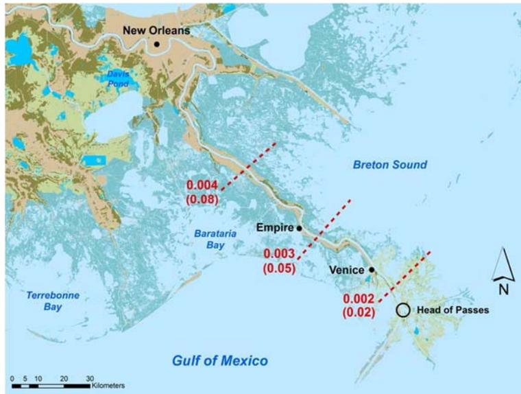
Figure 14. Recommended values for foreset slopes. Values in parentheses apply to sand size sediment.
