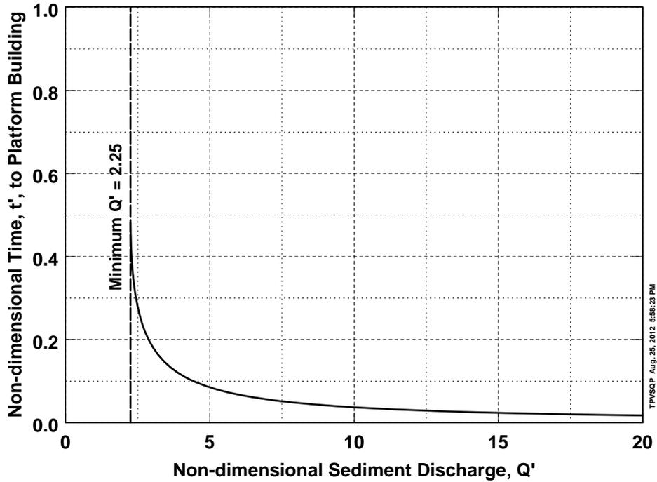
Figure B-1. Non-dimensional Time,  $t'$ , vs Non-dimensional Discharge,  $Q'$  for Truncated Cone.
