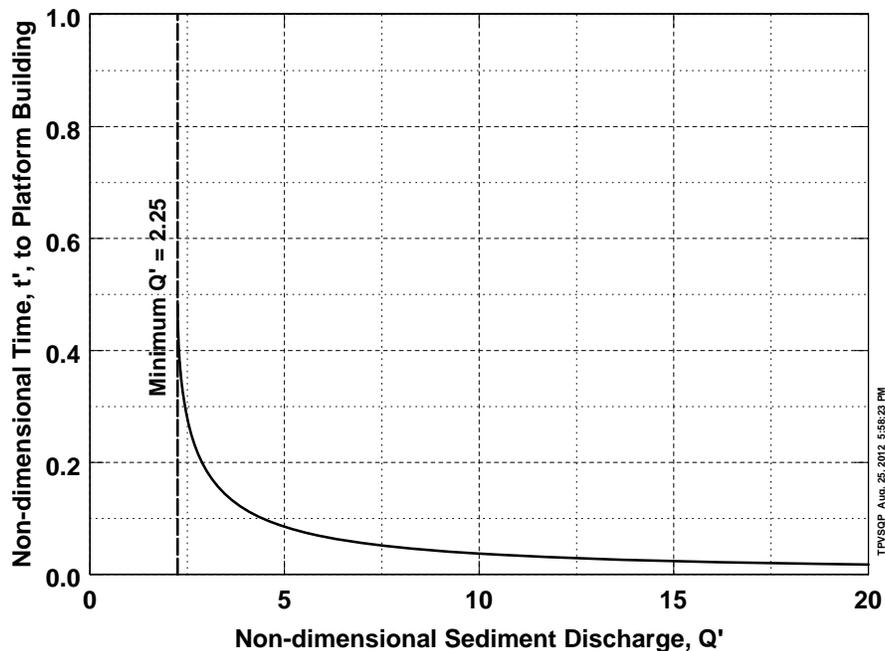
Figure 6. Non-dimensional time,  $t'$ , vs non-dimensional discharge,  $Q'$ , for truncated cone.
