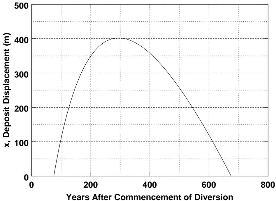
Figure 11. Example 3. Berm length,  $x$ , of deposit (see Figure 7) for diversion deposit of uniform width and into receiving waters of uniform depth. Annual volume of sediments retained = 60,000  $\text{m}^3/\text{year}$ , width of deposit = 2,000 m, initial depth = 1.5 m, elevation of deposit platform above water level = 0.25 m, relative sea level rise = 1 cm/yr.
