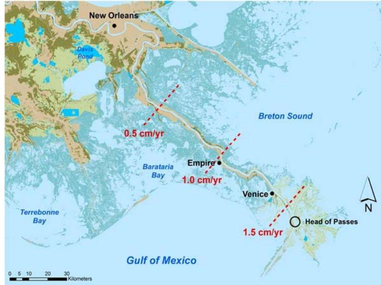
Figure 16. Preliminary recommendations for subsidence rates,  $F_s$ .
