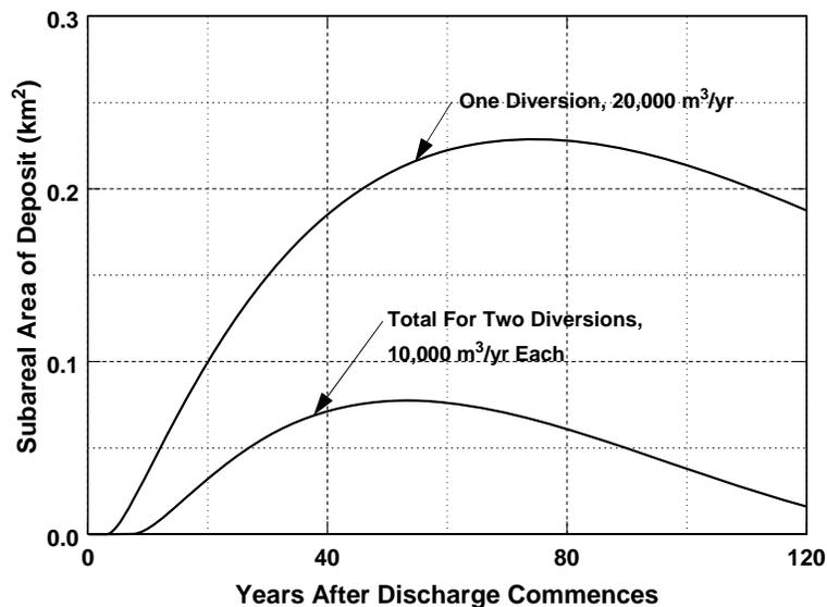
Figure 10. Example 2. Comparison of subaerial areas over time for one large diversion vs two diversions with the *same* total sediment retention. Initial depth of receiving waters = 0.75 m, elevation of horizontal portion of deposit above mean water level = 0.25 m, rate of relative sea level rise = 1.0 cm/yr, foreset slope = 0.002 and delta opening angle = 180°.
