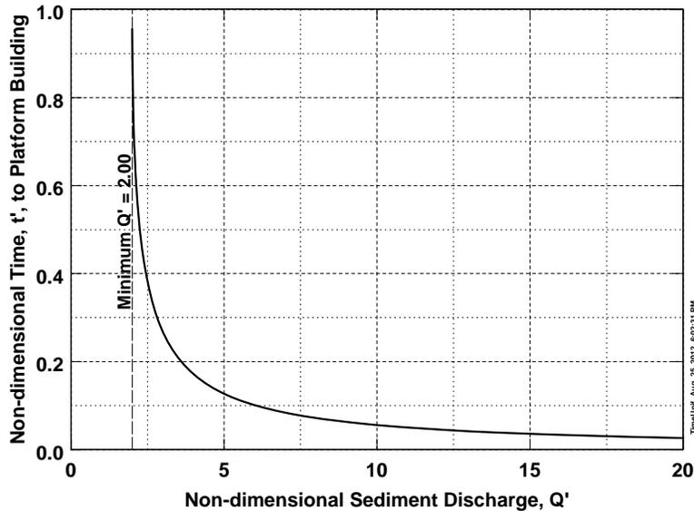
Figure 8. Non-dimensional time,  $t'$ , vs non-dimensional discharge,  $Q'$ , for uniform width and uniform depth model.
