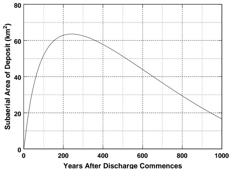
Figure 9. Example 1. Annual discharge of retained sediment =  $3 \times 10^6 \text{ m}^3/\text{yr}$ , initial depth of receiving waters = 2.0 m, elevation of horizontal portion of deposit above mean water level = 0.25 m, rate of relative sea level Rise = 2.0 cm/yr, foreset slope = 0.002 and delta opening angle =  $180^\circ$ .
