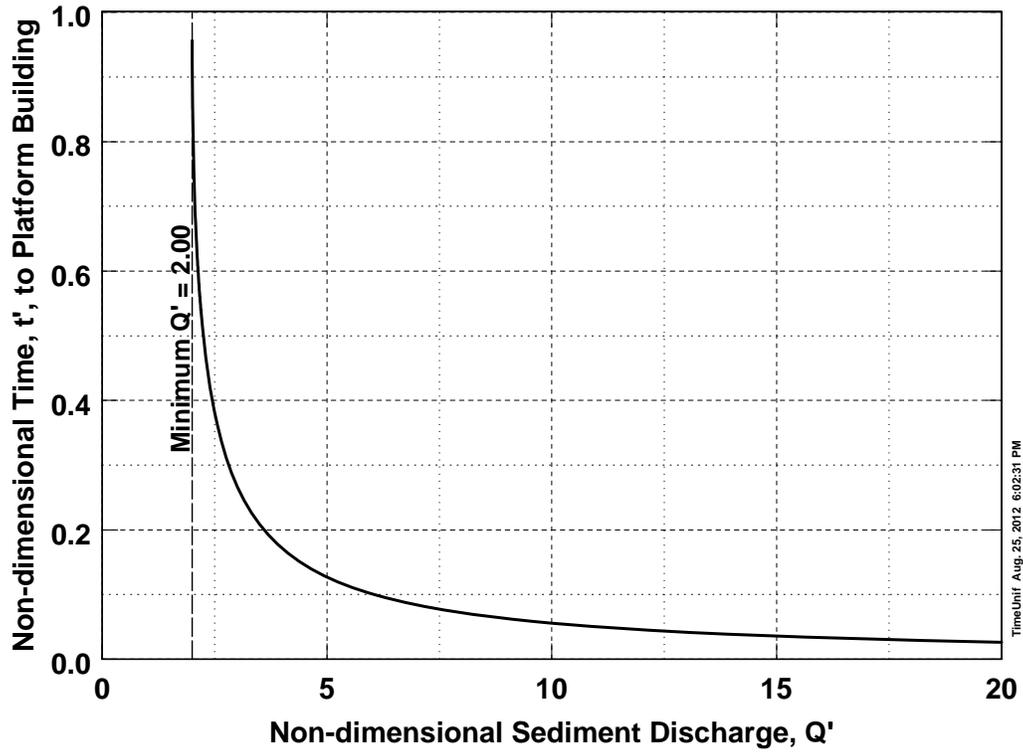
Figure B-2. Non-dimensional Time,  $t'$ , vs Non-dimensional Discharge,  $Q'$  for Uniform Width Model.
