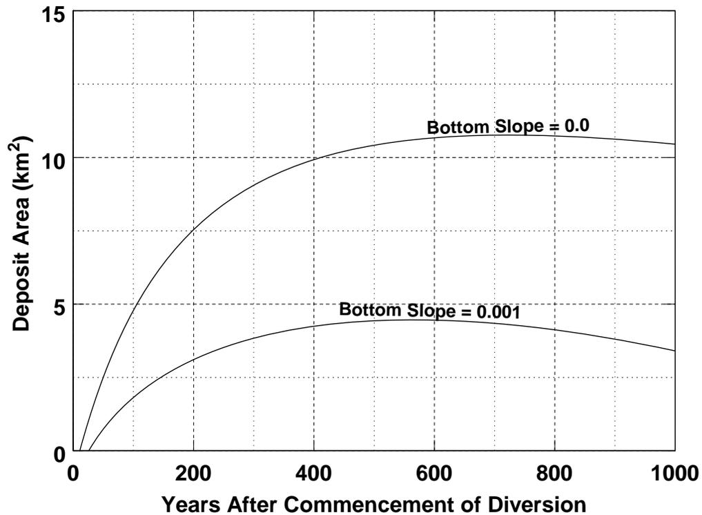
Figure 12. Example 4. Comparison of subaerial areas over time for two bottom slopes. Uniform width, annual retention of sediment = 200,000 m<sup>3</sup>/yr, relative sea level rise rate = 1.0 cm/yr. Initial depth of receiving waters = 0.75 m, Elevation of horizontal portion of deposit above mean water level = 0.25 m, foreset slope = 0.002.
