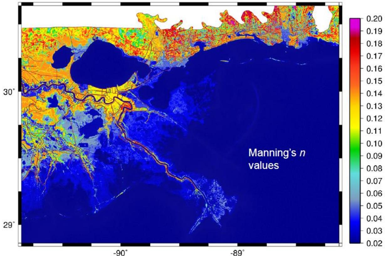
**Figure 5:** ADCIRC grid of Manning's  $n$  coefficient. (Source: Massey 2015.)
