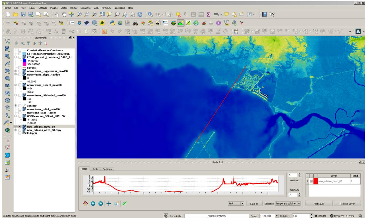
**Figure B.1:** Screenshot of the greater New Orleans digital elevation model along with the terrain profile tool spanning the northern tip of New Orleans East (Point aux Herbes) to the Pleistocene Terrace in Slidell. The red curve is the profile transect connecting the levee New Orleans East and to Slidell. The tool allows exporting the profile to a spreadsheet.
