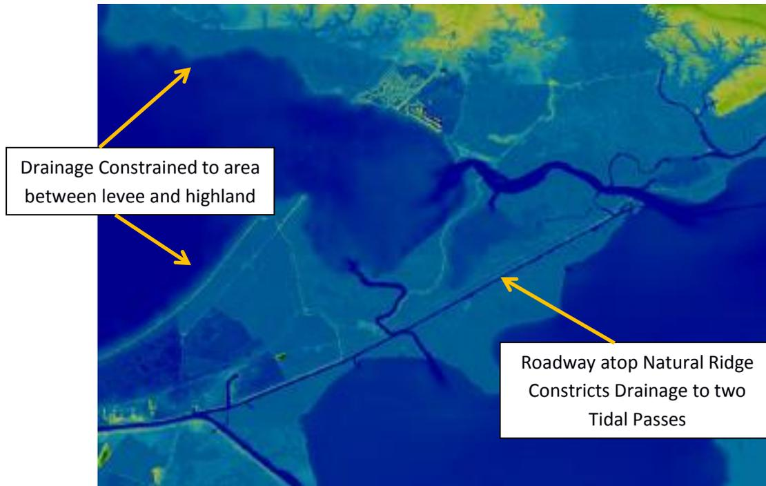
**Figure 33:** Storm surge outflow from Lake Pontchartrain is impeded by landscape features, such as the HSDRRS levee, and high ground on the north shore, The CSX railroad, the Hwy 90 roadbed atop the natural ridge. Once surge elevation lowers, outflow surge is limited to two tidal passes.
