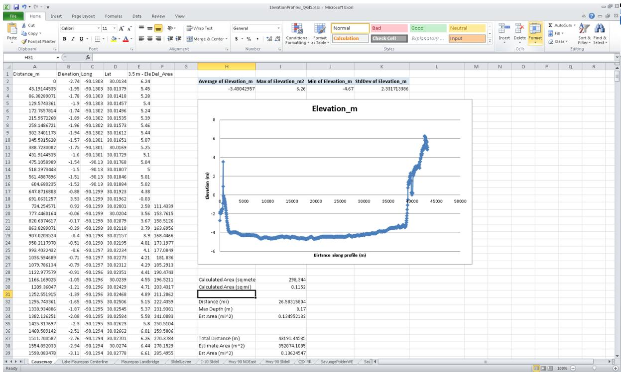
Figure B.2: Screenshot of terrain profile and cross-sectional area calculation.
