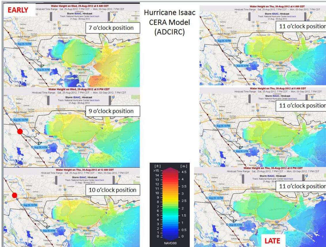
**Figure 12:** Snapshots from the ADCIRC surge model for Hurricane Isaac showing the peak surge rotating along the shoreline from the southwest banks toward the eastern banks in a counter clockwise direction. (orange-yellow=high surge; blue=low surge; red dot is eye of the hurricane) (Source: CERA.)
