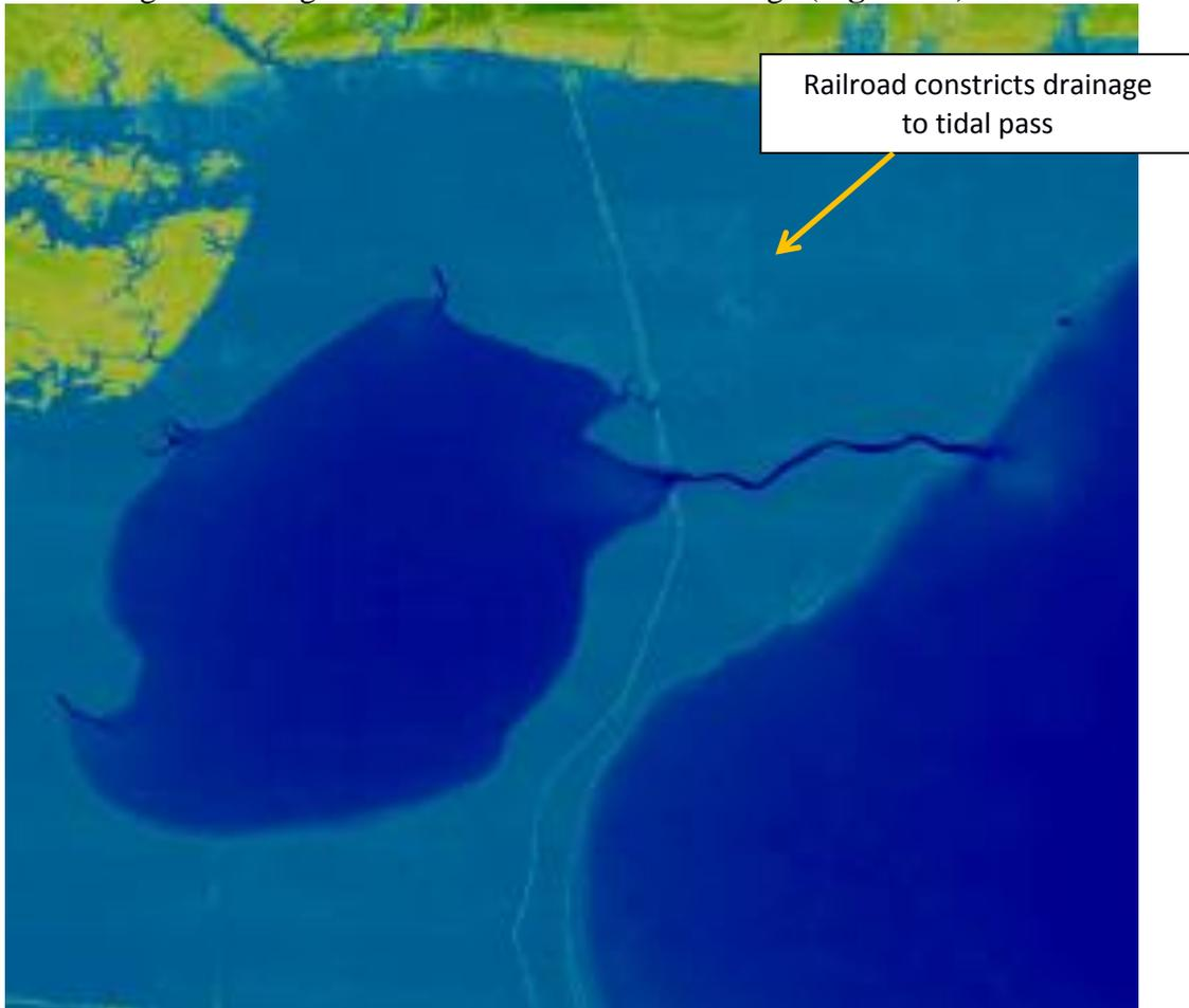
**Figure 32:** Once surge waters start to recede from Lake Maurepas, a railroad embankment atop the Maurepas Landbridge both acts as weirs. When the water levels drop below these terrain features, drainage is limited to Pass Manchac (Data Source: NOAA 2010).
