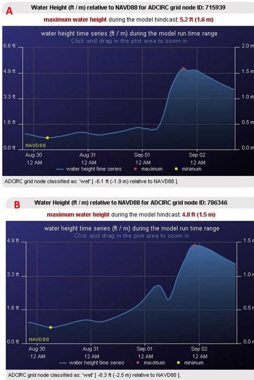
**Figure 28:** Simulated ADCIRC hydrographs from Hurricane Gustav from near the Mandeville gauge (A) and near the West End gauge (B). The fluctuation seen in the gauge hydrographs is also apparent in the ADCIRC results (Source: CERA.)
