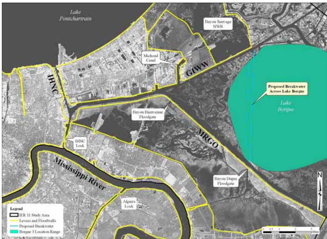
Figure 12 – Borgne 3 Location Range Alternative and Conceptual Layout for Storm Surge Protection Structures. Any breakwater built in the Borgne 3 Location Range would have to be used in conjunction with structures in the Borgne 1 or Borgne 2 Location Ranges to provide the 100-year level of protection.
