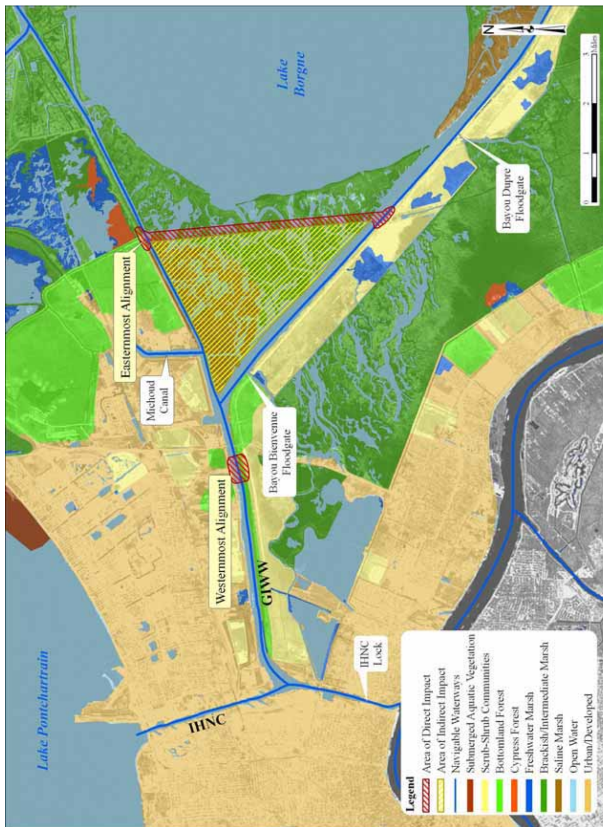
Figure 17—Area of Impact for Borgne 1 Alternative. This figure delineates the westernmost and easternmost possible alignments within Borgne 1 to show the minimum and maximum direct impacts to wetlands that could occur under proposed action.
