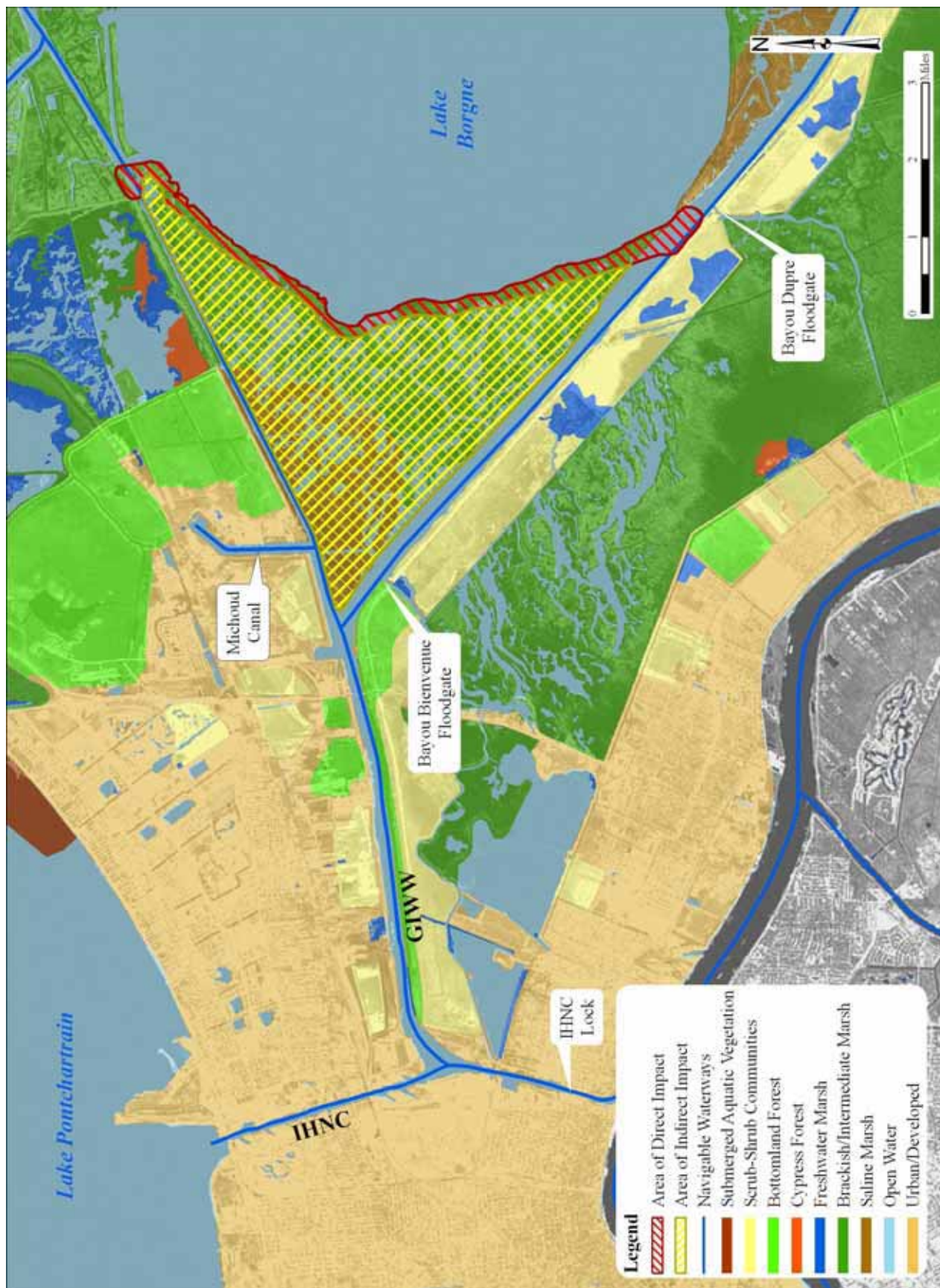
Figure 18 –Area of Impactfor Borgne 2 Alternative. The figure delineates the easternmost alignment to show the minimum possible impacts.
