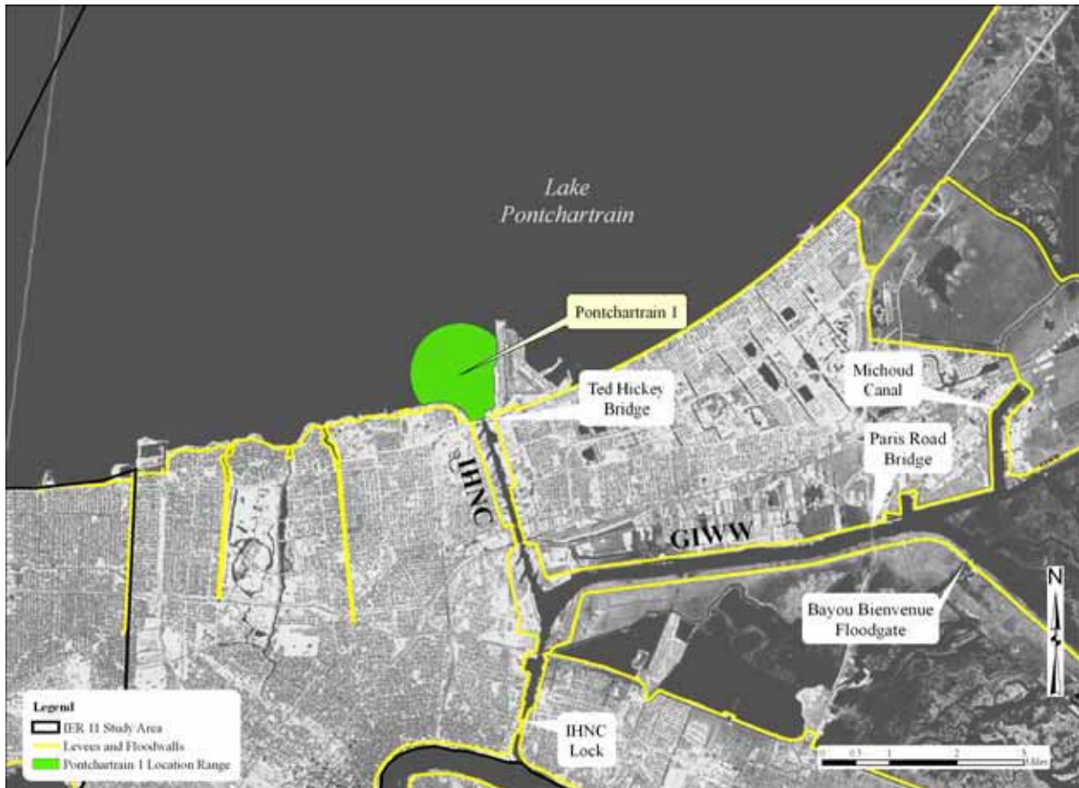
Figure 13 – Pontchartrain 1 Location Range for Storm Surge Protection Structure, extending from the Senator Ted Hickey Bridge approximately 1,000 feet north into Lake Pontchartrain.
