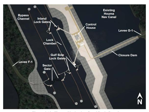
Figure 4-12. Houma Navigation Canal Lock Complex.
