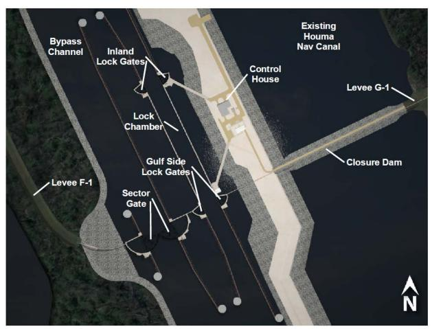
Figure 1-2. Houma Navigation Canal Lock Complex
