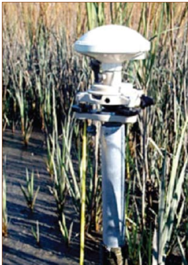
A continuously operating GPS reference station, part of CORS
