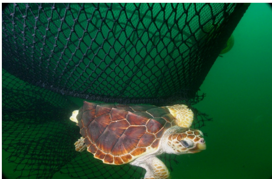
Figure 5.5-6. A loggerhead sea turtle escapes from a trawl equipped with a turtle excluder device (TED) during TED testing. TEDs are used to reduce bycatch of sea turtles in trawl nets.
