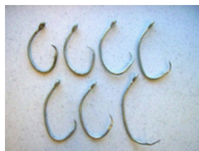
Figure 5.D-18. Standard circle hooks (top) and weak circle hooks (bottom) after bluefin tuna experiments.
