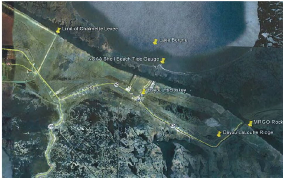
Figure 2.12. Area east of the LPV flood protection system along Bayou Yscloskey and the Bayou LaLoutre ridge, showing location of MRGO Rock Dam where the LaLoutre Ridge was bisected by the MRGO.
