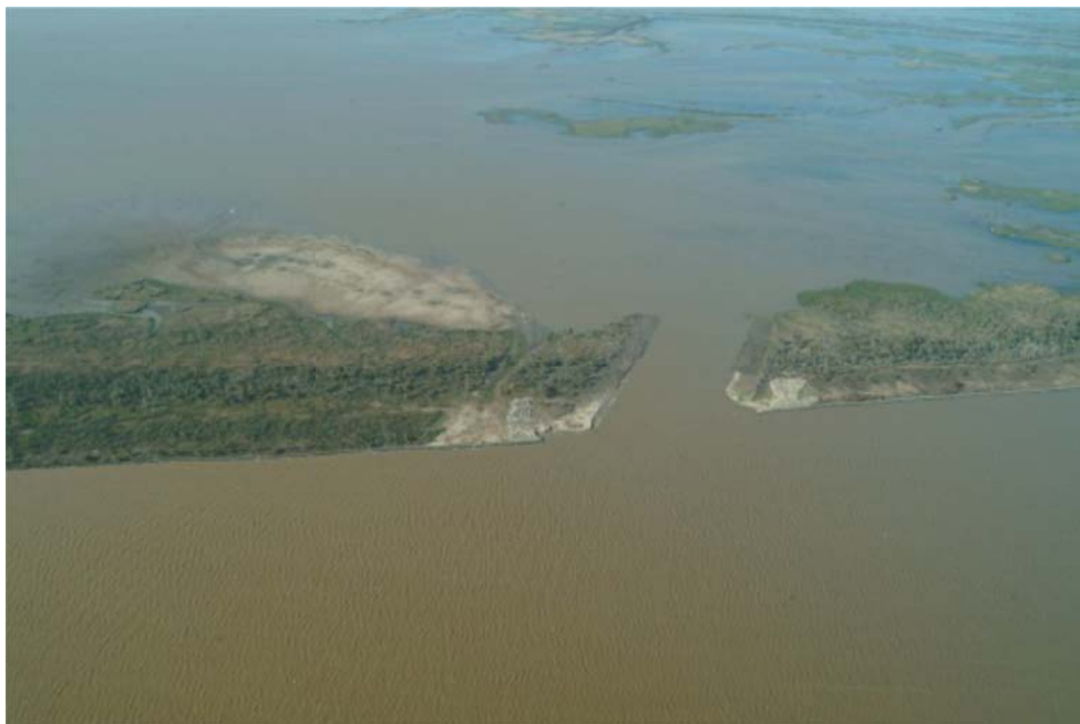
Figure 1-5. Photo of West Bay Diversion (20,000 cfs capacity) The Breaux Act Task Force voted to close West Bay. [from Louisiana Coastal Wetlands Conservation and Restoration Task Force 2004 (rev.)]
