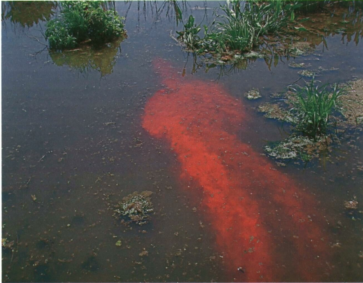
Figure 6. Movement of tracer dye through the water at the Hammond assimilation wetland.
