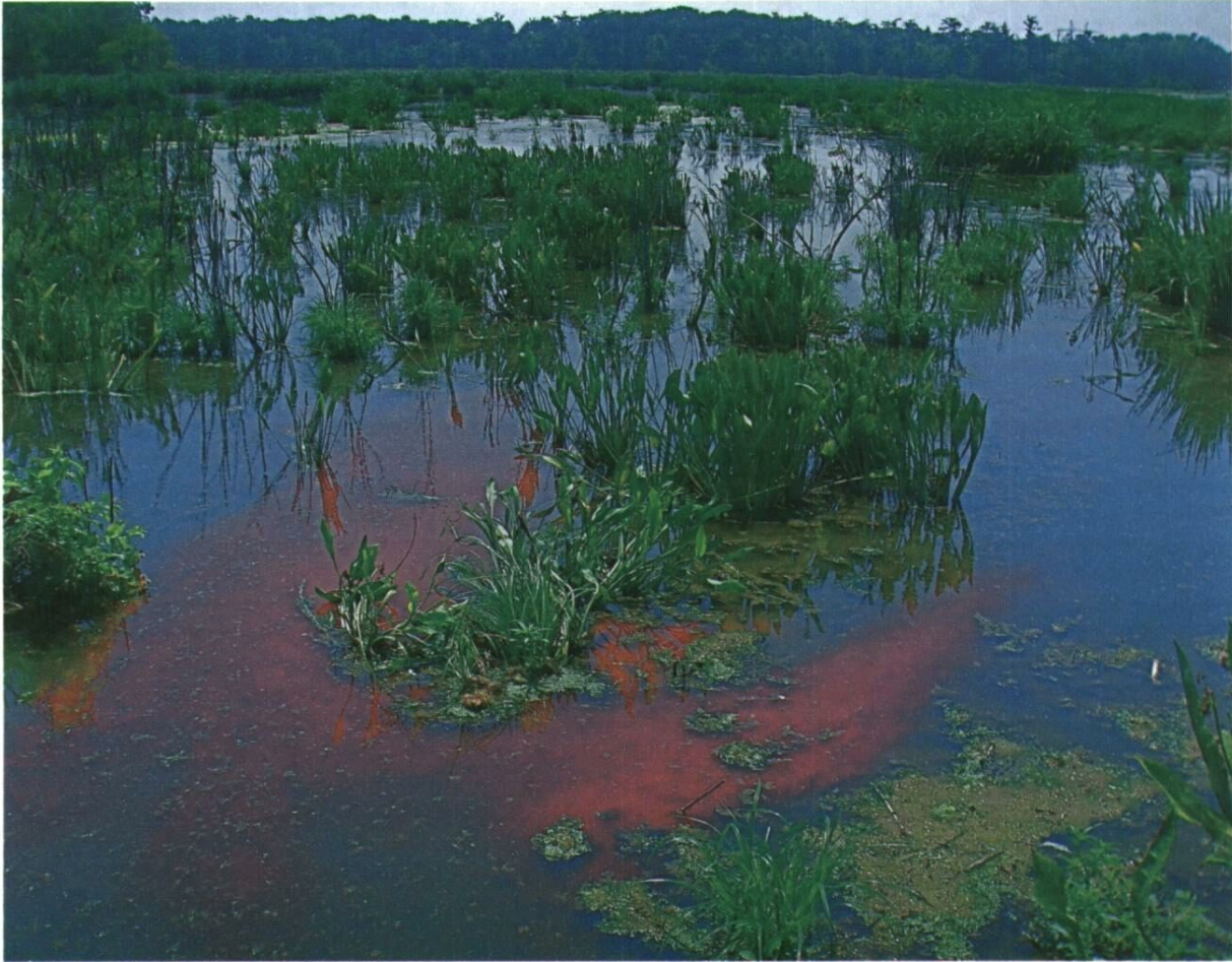
Figure 7. Movement of tracer dye through the water at the Hammond assimilation wetland. Note how dye moves around vegetation.
