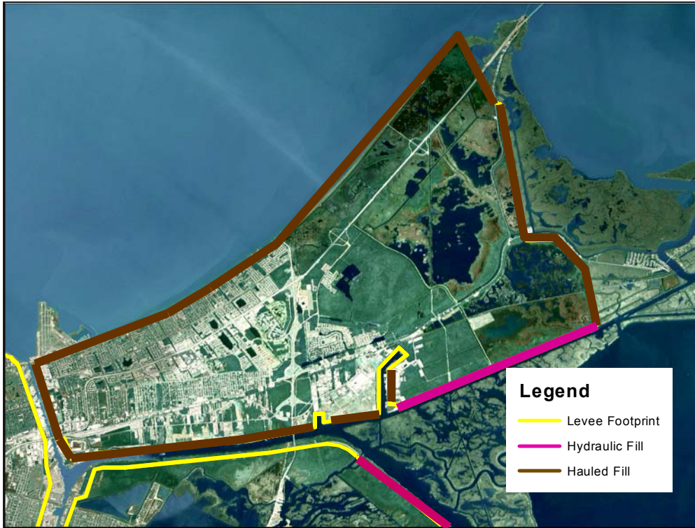
Figure 21a. Character of levee materials, New Orleans East and northern St. Bernard. This slide is incomplete for St. Bernard and shows only the hydraulic fill section along the MRGO.
