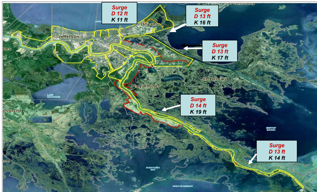
Figure 16. Comparison of general surge levels assumed in the SPH design (D) and estimated from Katrina (K). See Volume IV for more detailed information.
