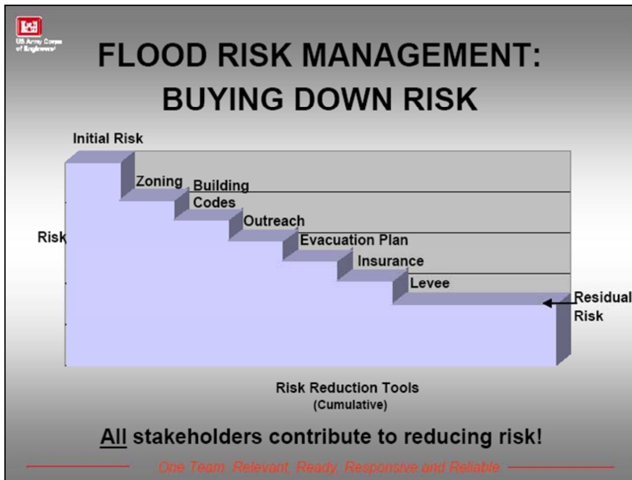
Figure 1. Illustration of residual risk and risk reduction measures. Source: U.S. Army Corps of Engineers.
