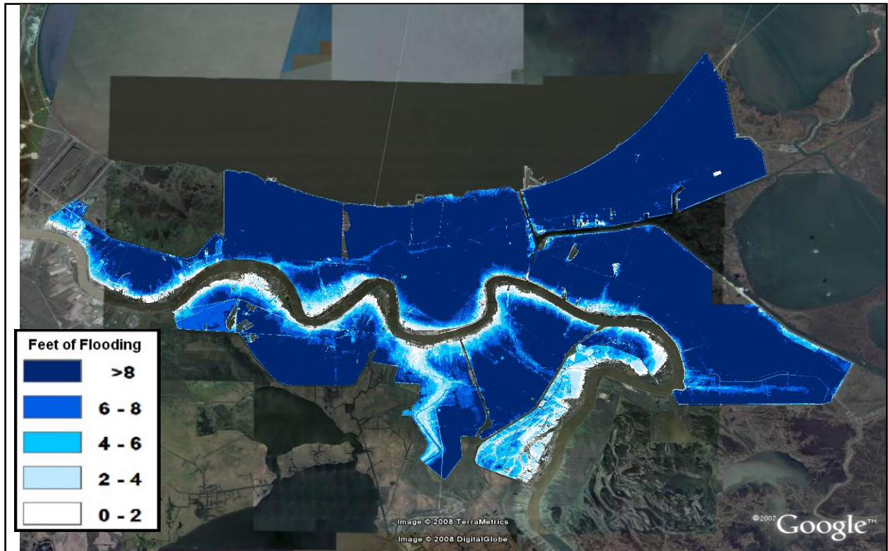
Figure 10-17. Hurricane inundation frequency map, 0.2% (1/500 return period) for pre-Katrina HPS and 100% of ideal pumping.
