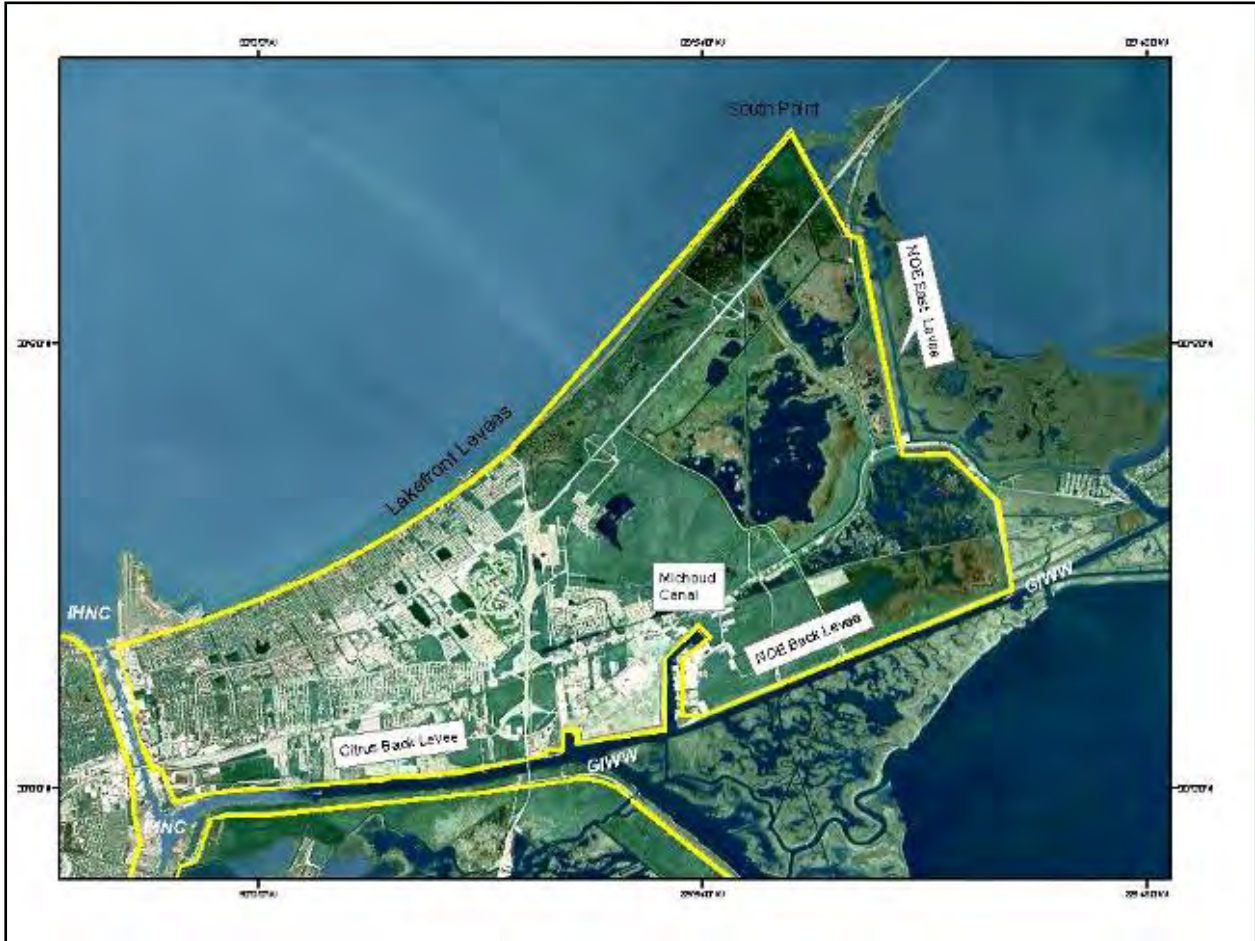
Figure 63. General Map of NOE Basin, Major Levee Segments are Lakefront Levees, NOE East Levee (South Point to GIWW), NOE Back Levee, Citrus Back Levee, and IHNC Levees
