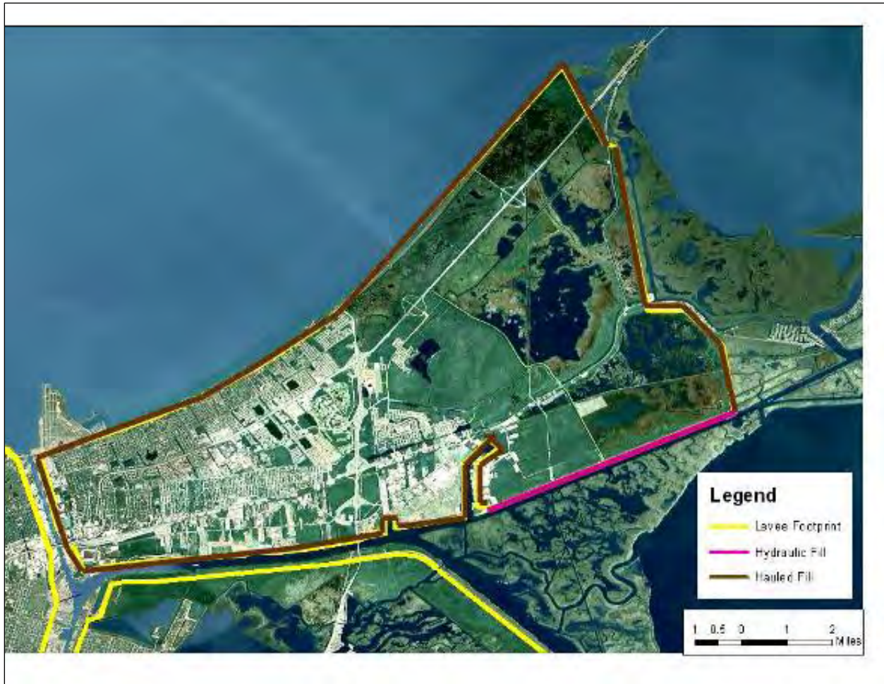
Figure 65. NOE Levee Construction Materials (USACE DM NOE Back Levee, Citrus Back Levee, South Point to GIWW Levee, Lakefront Levees, and IHNC Levees) 1971, 1969, etc.)
