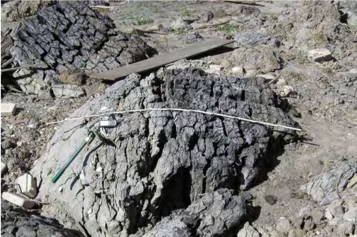
Figure 9. Clay Attached to Marsh Blocks at the 17th Street Canal Breach
