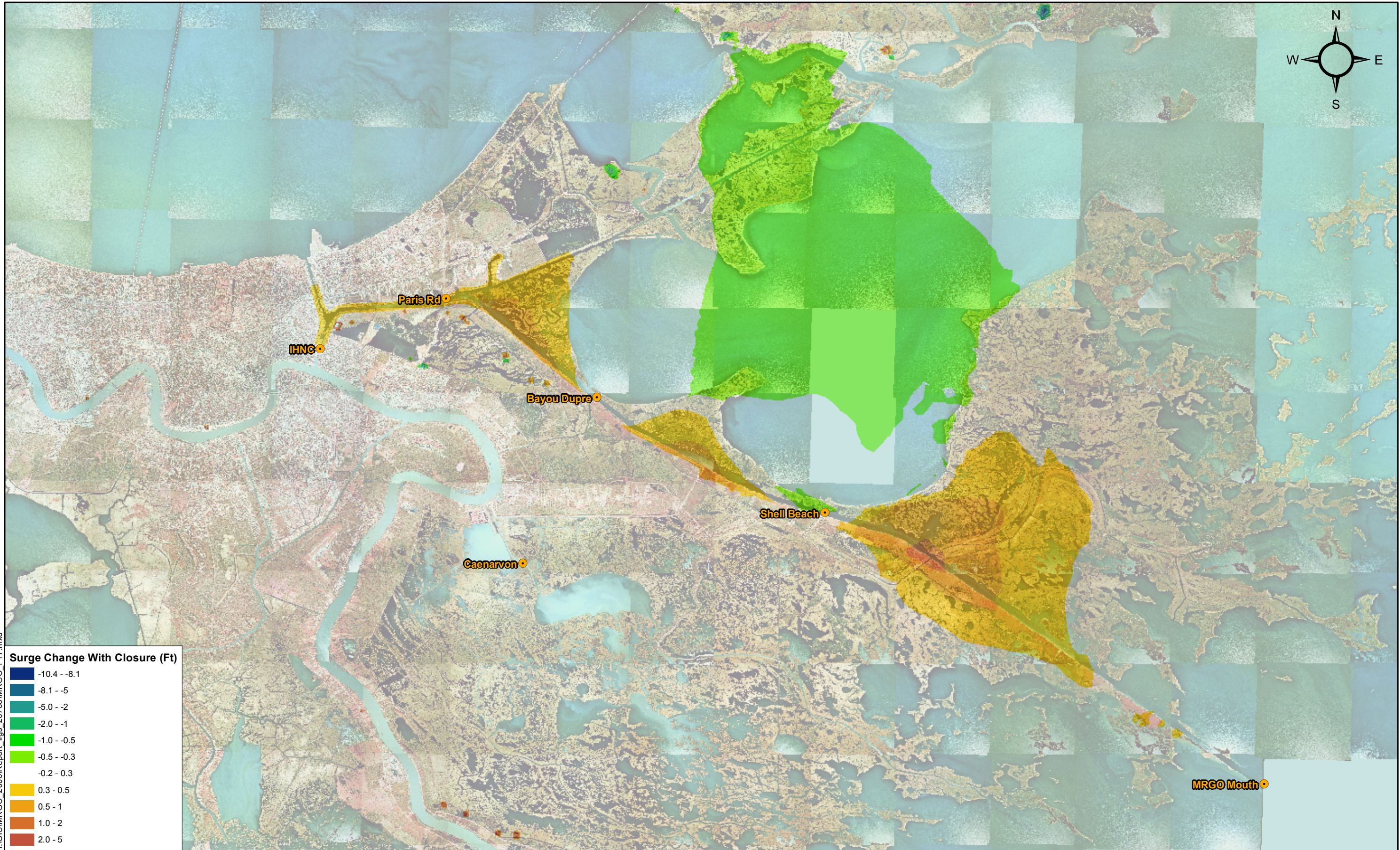
Figure 17 Difference in Maximum Water Surface Elevation for Hurricane Betsy, Baseline vs. Closed MRGO
