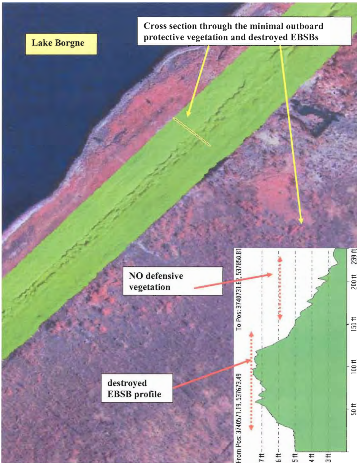
Figure 46: Processed LiDAR post-Hurricane Katrina survey data showing NO defensive line of vegetation outboard of the MR-GO Reach 2 EBSBs and the breached profile of the EBSBs in this section of the alignment (Morris 2008).
