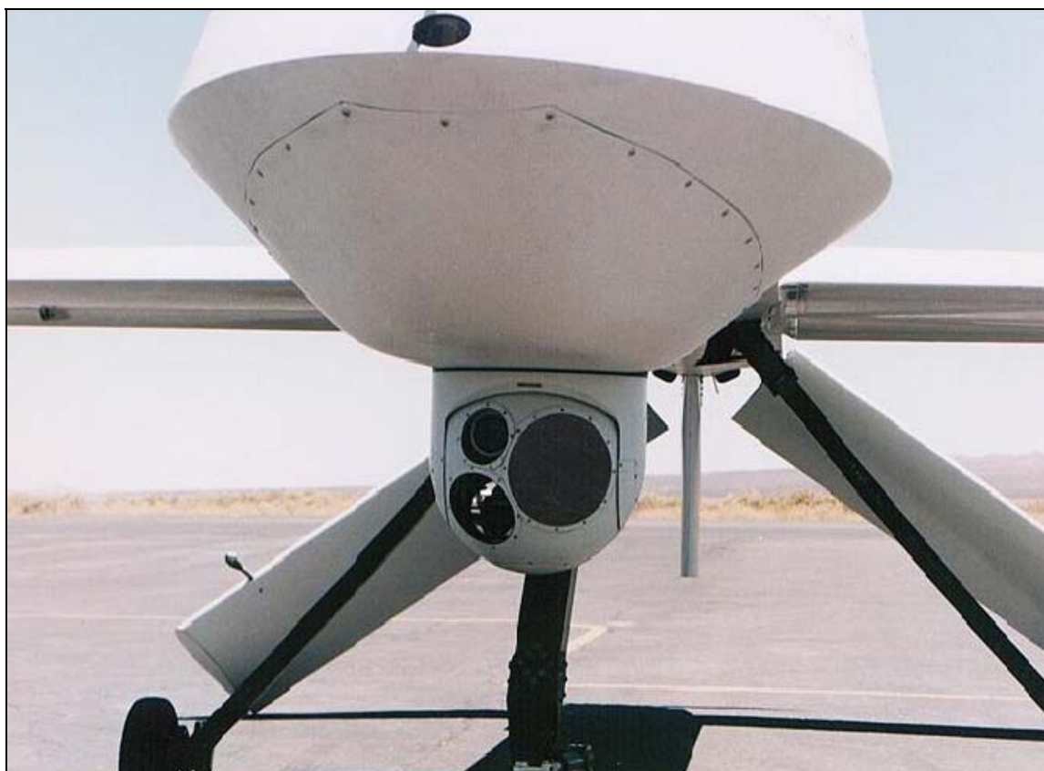
Figure 2. An Electro-Optical/Infrared (EO/IR) Sensor Housed in a Pod Mounted on an MQ-9 Predator B/Reaper Drone Operated by Customs and Border Protection (CBP)
