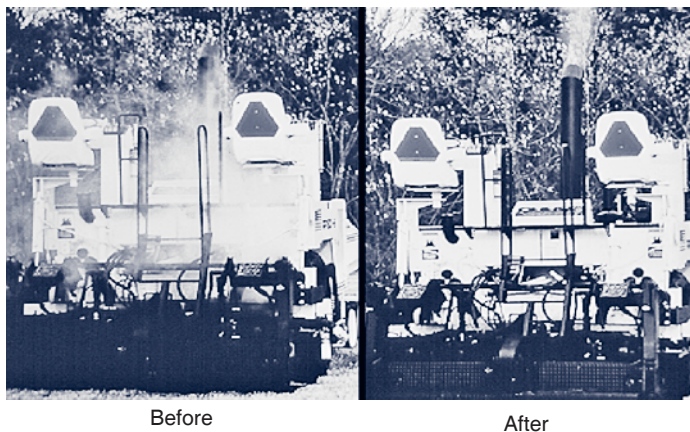
FIGURE 1. Asphalt paver before (left) and after installation of an engineering control to reduce exposures to asphalt fumes
