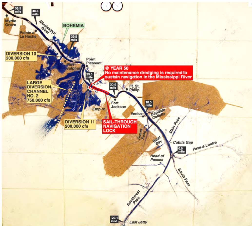
PHOTO NO. 9: LARGE DIVERSION CHANNEL NO. 2 State of Sedimentation after 50 years of operation
